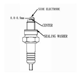
Too large gap, deposit and electrode erosion will result in incomplete spark.
